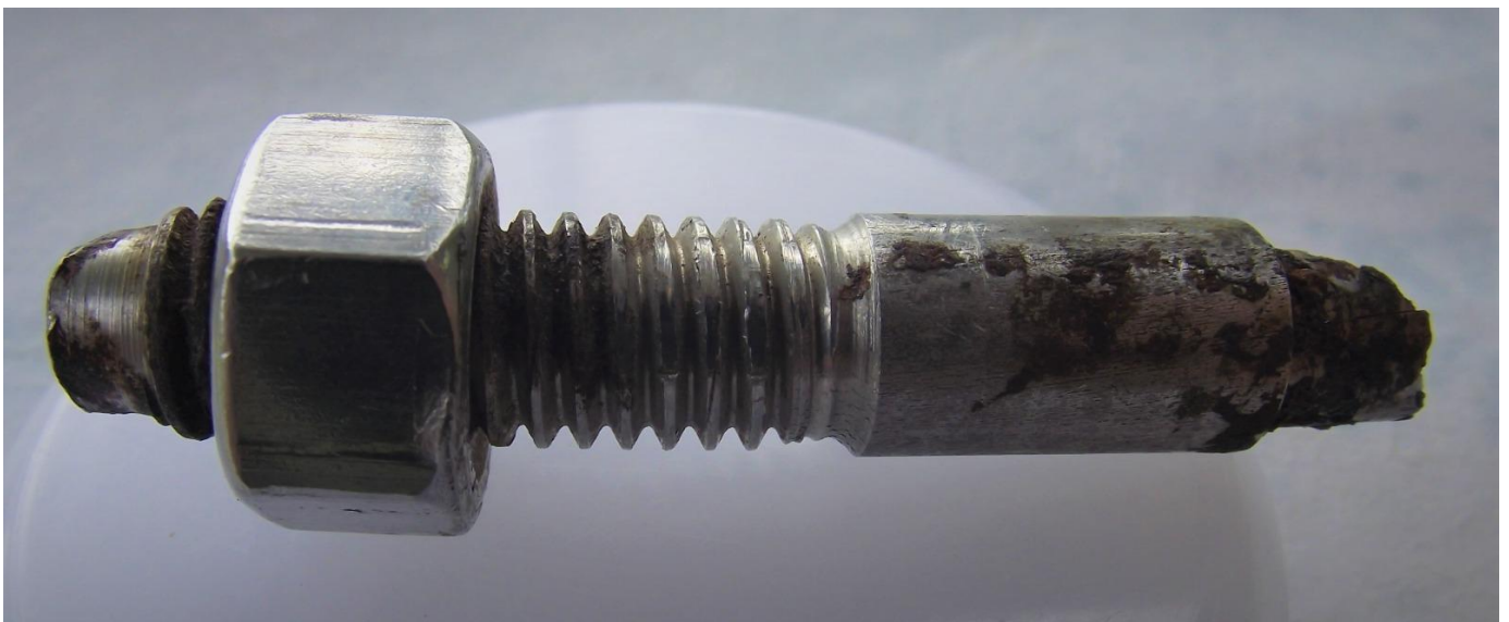
Figure 1 - Failed anchor bolt analyzed, Sample
